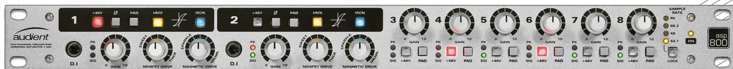
Channels 1 & 2 each offer different tone shaping via HMX and IRON circuits.
